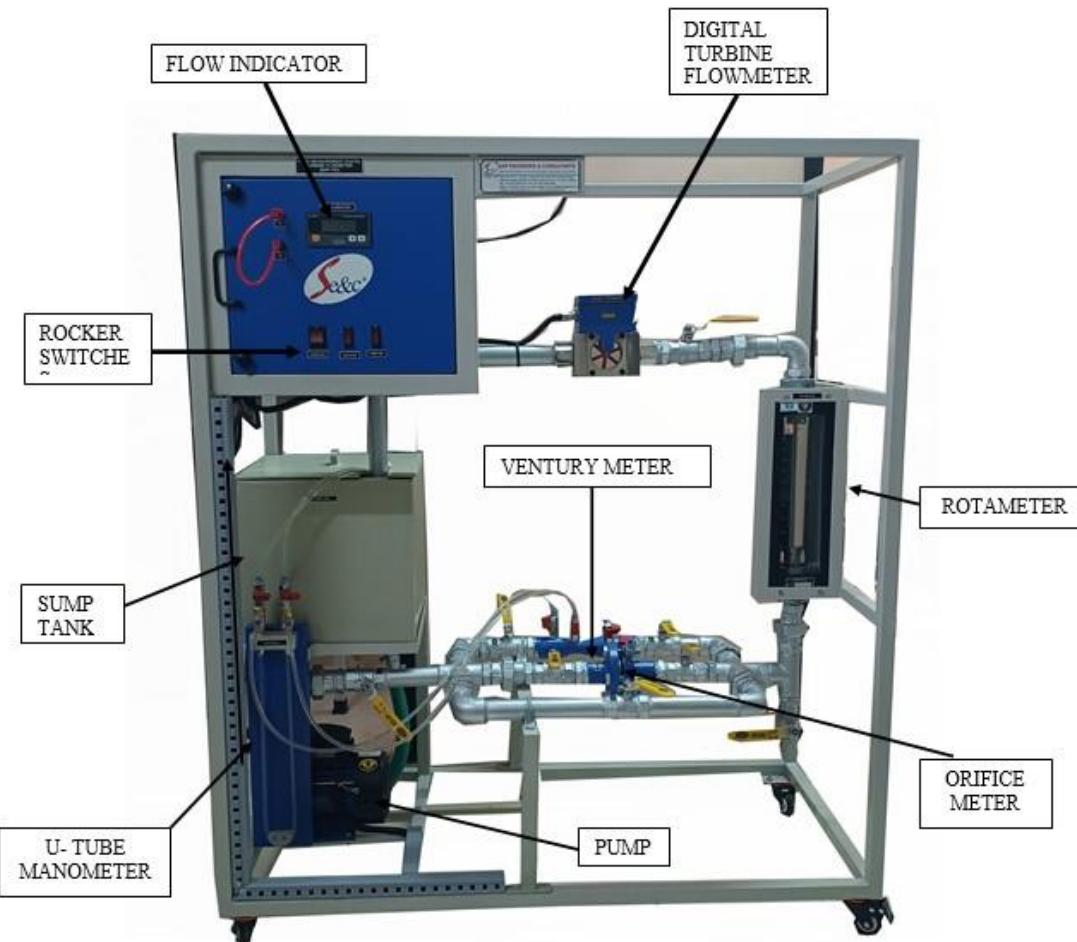
The **Setup for Calibration of Flow Sensor (SAP – 15D)** gives an idea regarding Flow Sensor & Flow Transmitter Principle. It outlines the procedure for calibration of flow Sensors/Transmitters.
